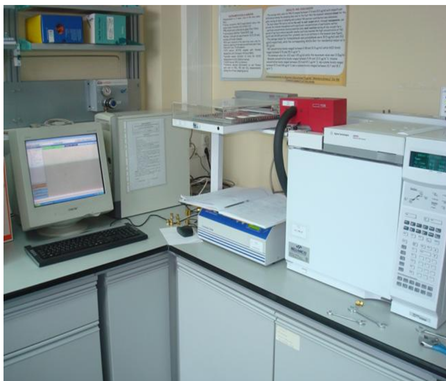
Agilent Technologies 7890A GC System coupled with Gerstel Thermal Desorption System, FID Detector
